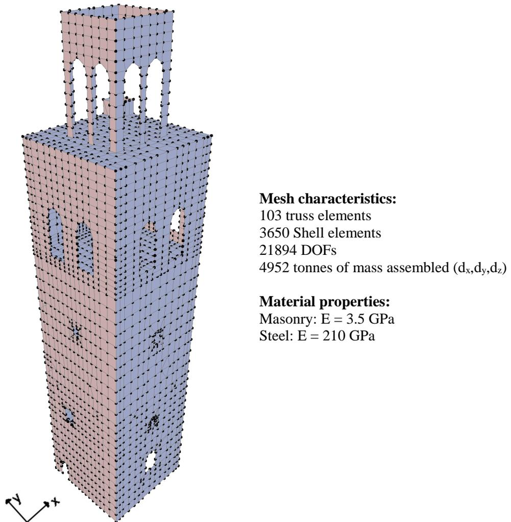
Figure 5 Numerical model characteristics
