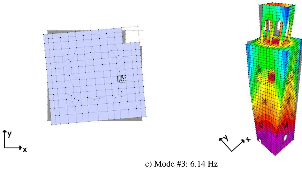
**Figure 6** Numerical mode shapes
