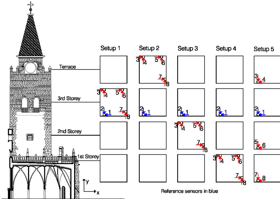
Figure 2 Experimental Test Setups
