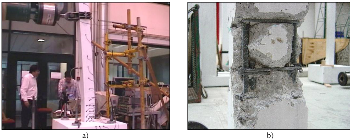
Figure 3.4. Monotonic test with specimen P1 performed by Mendes et al. (Mendes et al. , 2007): a) test under execution; b) inspection made to the reinforcements after the test.
