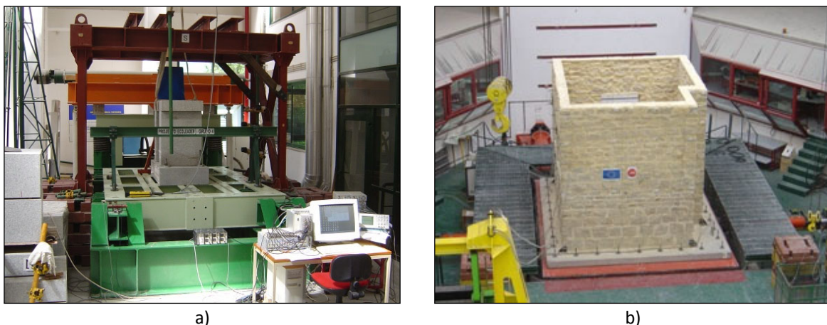
Figure I.4: Large-scale seismic testing facility at LNEC: a) Uniaxial shaking table; b) Triaxial shaking table.
