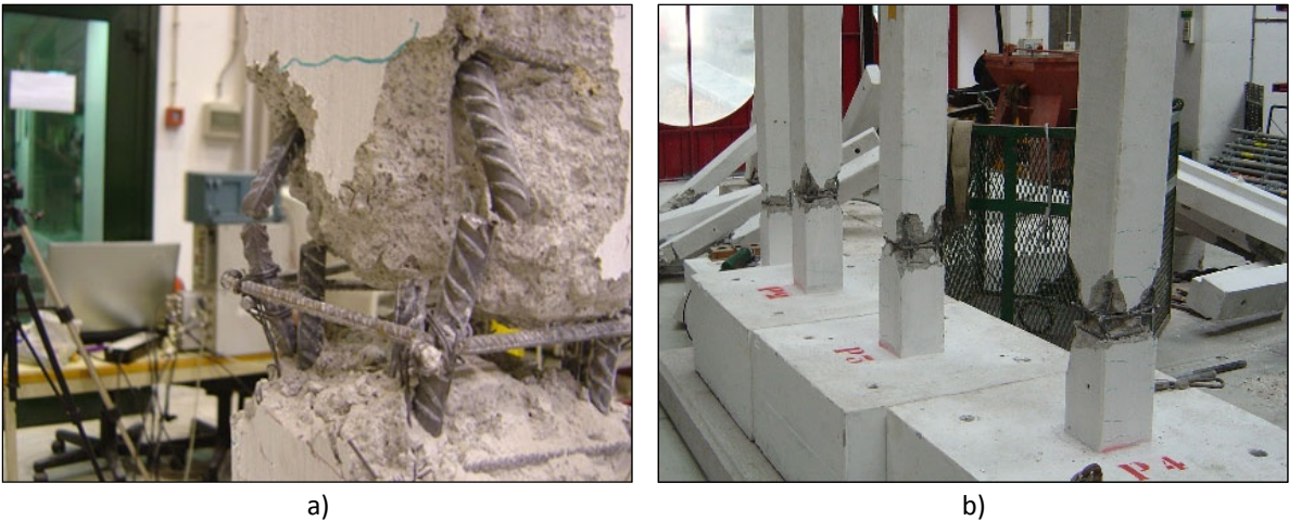
Figure III.133: Example RC4 – Specimens after the testing: a) Specimen P4 after inspection; b) General view of the four column-foundation specimens.
