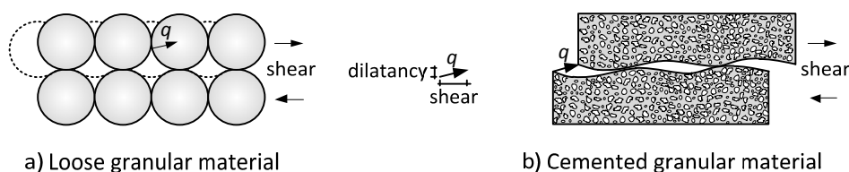
Figure III.2: Dilatancy phenomenon for granular materials, adapted from Vermeer et al. [556].
